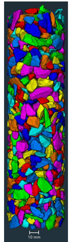
Figure 2. CT of aggregates.
