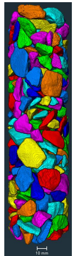
Figure 2. CT of aggregates.
