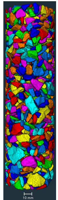
Figure 2. CT of aggregates.
