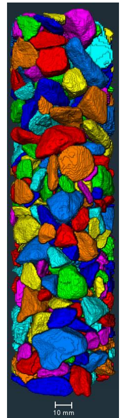
Figure 2. CT of aggregates.
