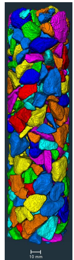
Figure 2. CT of aggregates.
